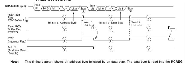
This timing diagram shows an address byte followed by an data byte. The data byte is read into the RCREG (Receive Buffer) because ADEN was updated after an address match, and was cleared to a '0', so the contents of the Receive Shift Register (RSR) are read into the Receive Buffer regardless of the value of bit 8.
