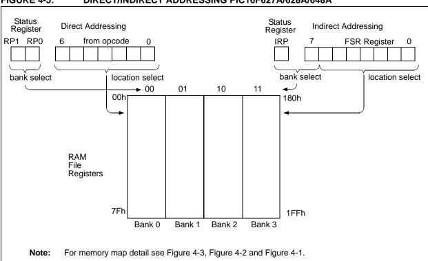
FIGURE 4-5: DIRECT/INDIRECT ADDRESSING PIC16F627A/628A/648A
