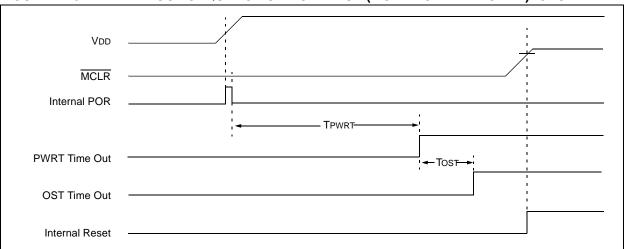
FIGURE 14-10: TIME OUT SEQUENCE ON POWER-UP (MCLR TIED TO VDD)
