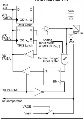
FIGURE 5-3: BLOCK DIAGRAM OF THE RA3/AN3/CMP1 PIN
